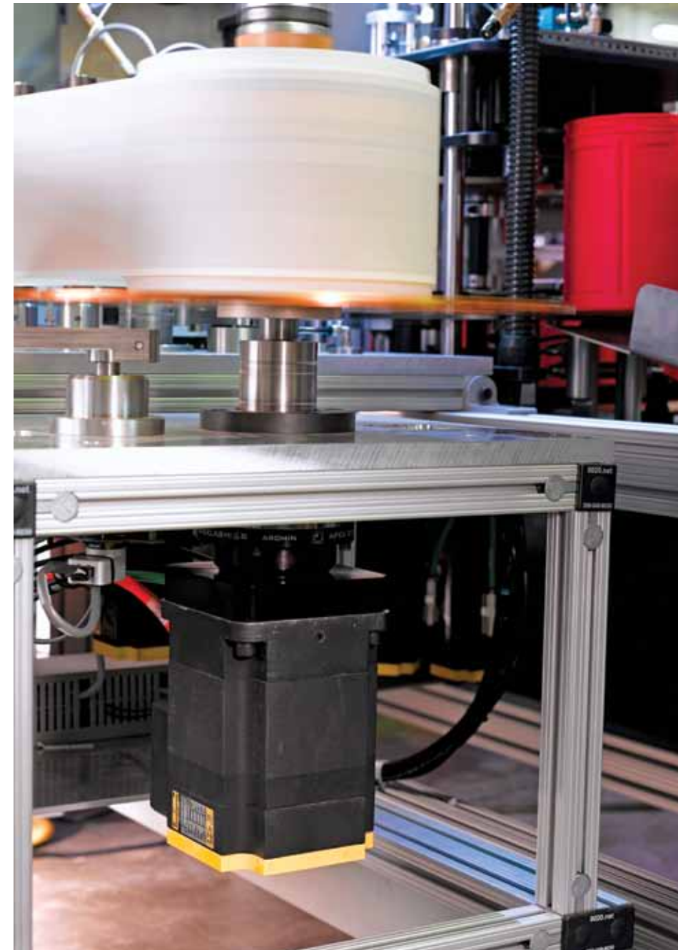
Baldor motion control products are programmed to provide the right feed, placement and pressure for the machine to apply heat transfer labels from a preprinted, continuous paper web to the container. This new equipment has helped the end user become more efficient by taking its scrap rate of 7% at 50 containers per minute to less than half of 1% at 60 containers per minute.
