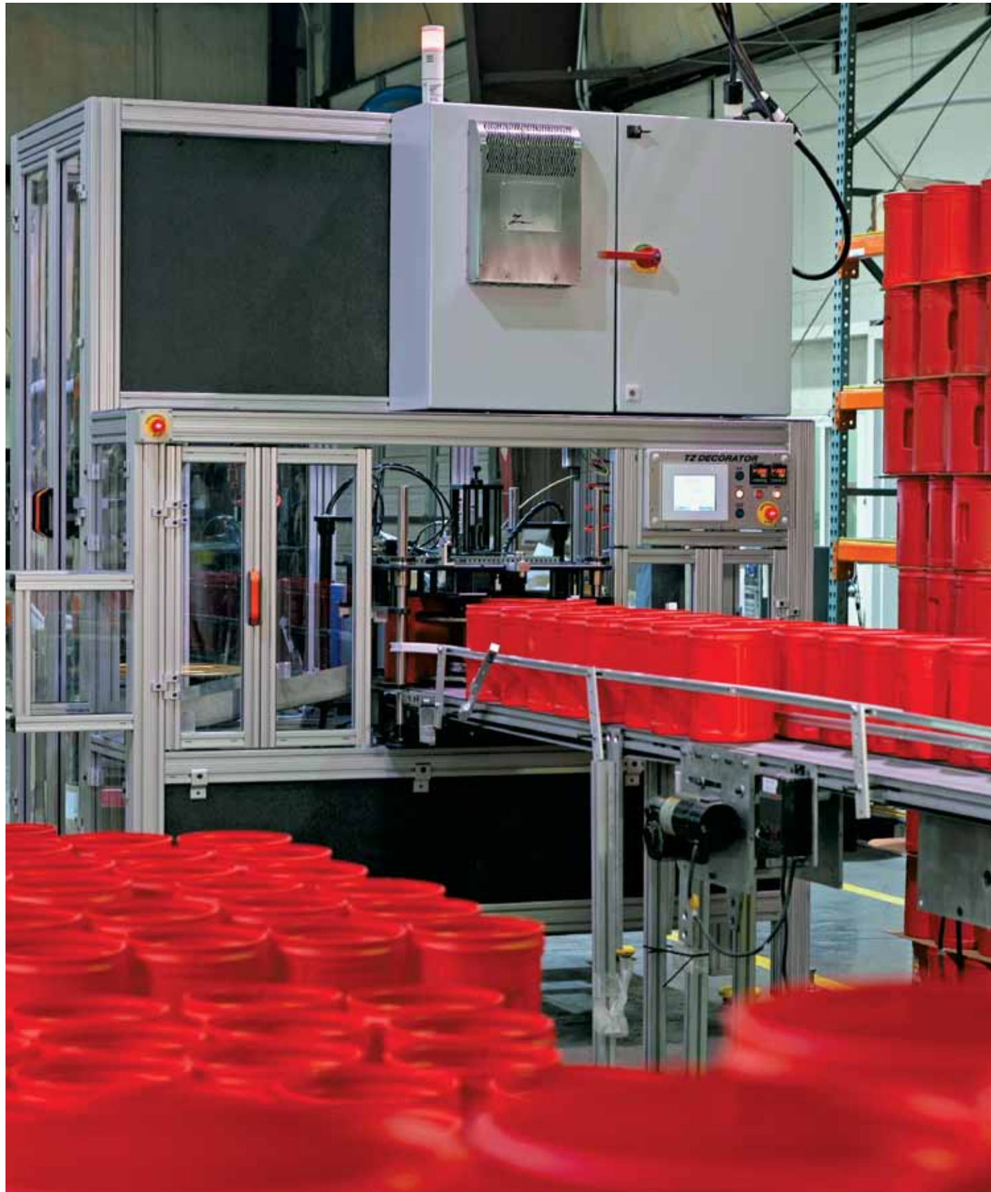
This high-speed labeling machine is designed for a unique heat-transfer decorating process for plastic containers. Baldor motion control products were selected because of the power, reliability and flexibility they provide. Coupled with Baldor's Mint® easy-to-use programming language, the system captures, orients and presents containers to the labeling heads for accurate label placement.
